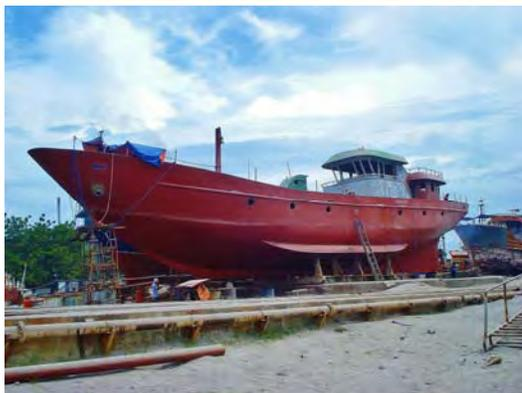
The photo to the right shows her portside stern. Primer painting of the deck structure is underway in this picture. You will notice as well what appears to be five vertical lines at the fantail. This indicates additional welding we required the shipyard to accomplish on the stiffeners in the steering gear room. All the windows and doors for the deck structure have been fabricated and were ready for installation here, however we also required x-bracing to be welded into place to prevent twist.
