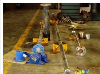
Propeller shafting, couplings, pedestal bearings and the new propeller are all shown in this photo inside the machine shop of SAFI Shipyard.
