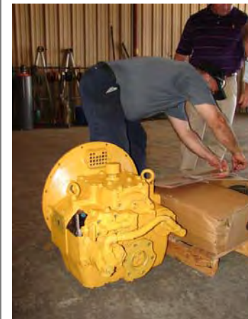
The Twin-Disc hydraulic reduction gear (marine transmission) provided by Sewart Supply, Morgan City, Louisiana.
