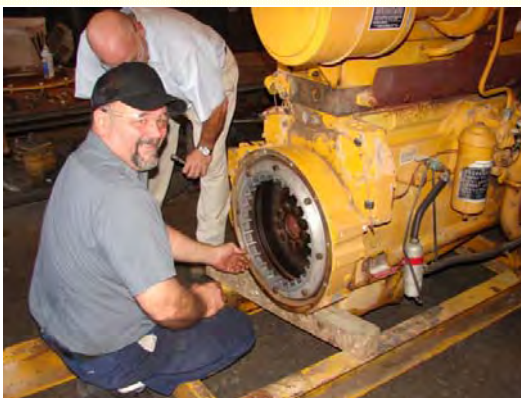
The photo above shows the ring-gear being bolted onto the engine's flywheel by Glen, one of the mechanics at Sewart Supply.
